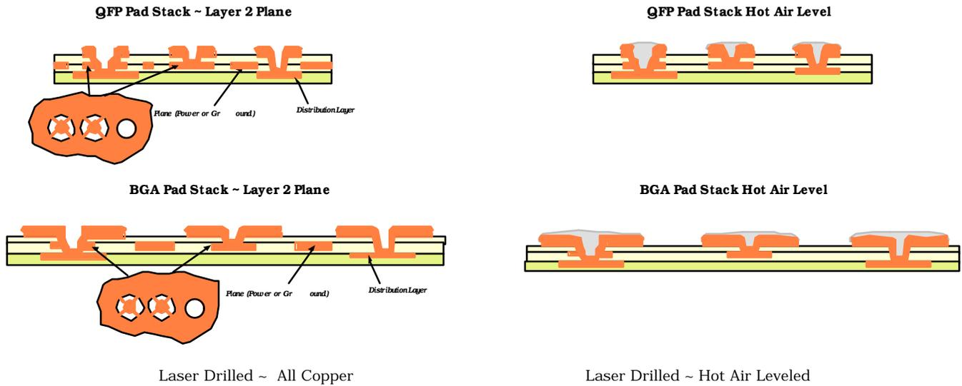
Laser Drilled ~ All Copper
