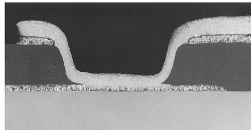
Laser Drilled Blind Via ~ 1985
