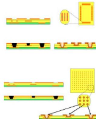
The limitation of these multi-depth laser drilled blind vias is the ability of the fabricator to plate into the blind vias. The finished board may be all copper or hot air leveled as shown below:
