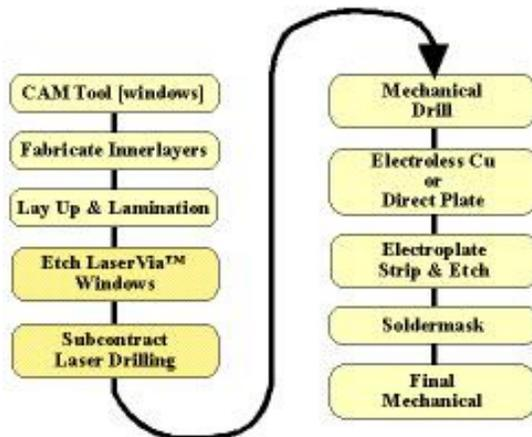
*Process Flow Diagram - Foil Lamination*
