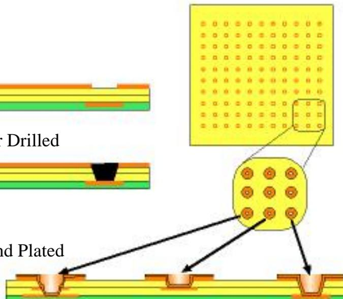
Most circuit board wet processing lines can plate a 1:1 ratio (diameter to depth) blind via. Since gas entrapment can inhibit blind via plating in the electroless line, a “bump or thump” of the agitation racking system can readily jar gas entrapped bubbles from the blind vias assuring continuous plating.
