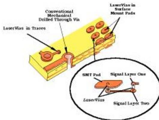
One solution for the “Interconnection Gap” is blind via technology and the best blind via solution is Via-in-Pad interconnections.
