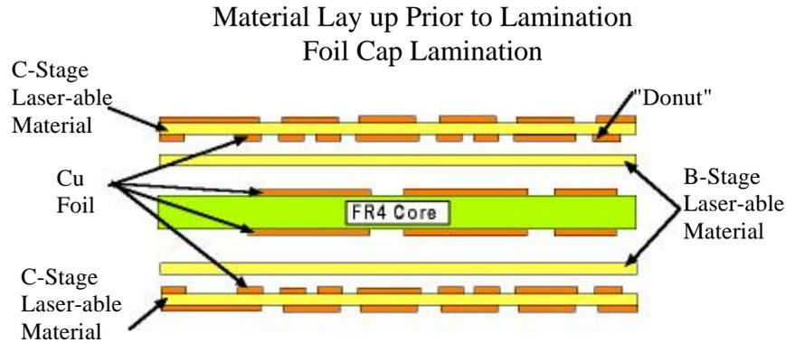
2. Foil Cap Lamination: a thin core is used for the outer layer with a laser-able prepreg between circuit layers two and three.
