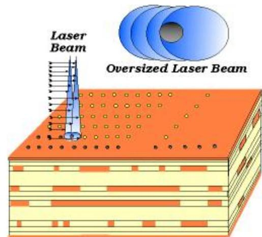
As laser drilling and fabrication processes mature (etching, plating etc.), narrow deep blind via interconnects will emerge to levels as deep as four layers down.
