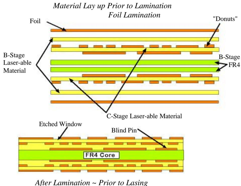
The preferred lamination process for multi-depth laser drilled blind vias fabrication is Foil Cap Lamination since the alignment of the outer windows and layer two donuts are imaged and etched at the same time. Using a typical inner layer registration technique for etching the outer windows and inner layer donuts relieves the problems that characteristically occur with material movement and “blind” registration to the layer two donuts.
