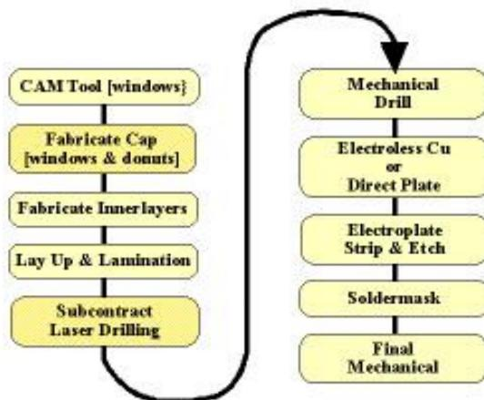
*Process Flow Diagram - Foil Cap Lamination*
