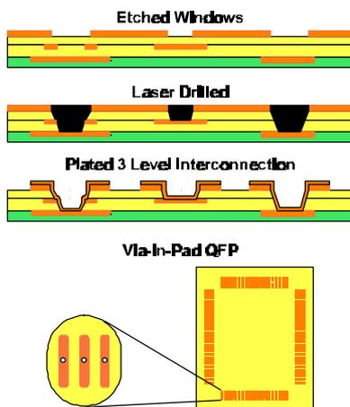
**Fig. 8 QFP Multi-Level Interconnections**
