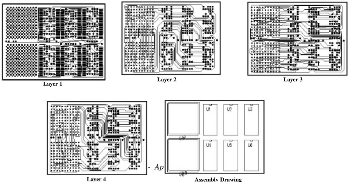
**Fig. 3 Routing Layers Through Via Design**
