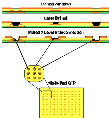
**Fig. 7 BGA Multi-Level Interconnections**
