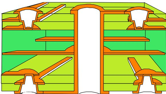
**Fig. 2 Three Level Laser Drilled Blind Vias**
