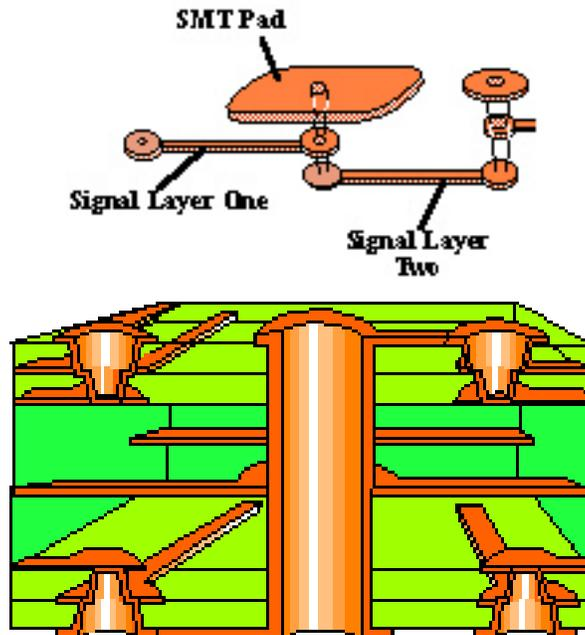
Figure 4. "Multiple Depth" Microvias
