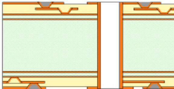
*Figure 6. Buildup Technology "Staggered Vias"*
