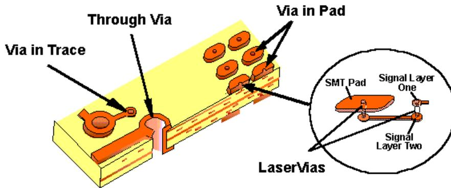
Figure 3. "Single Depth" Microvias
