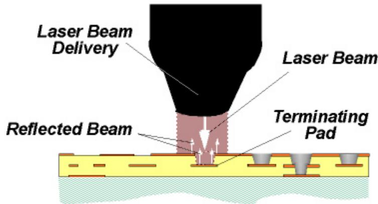
Figure 1. IR Laser - Reflected Beam
